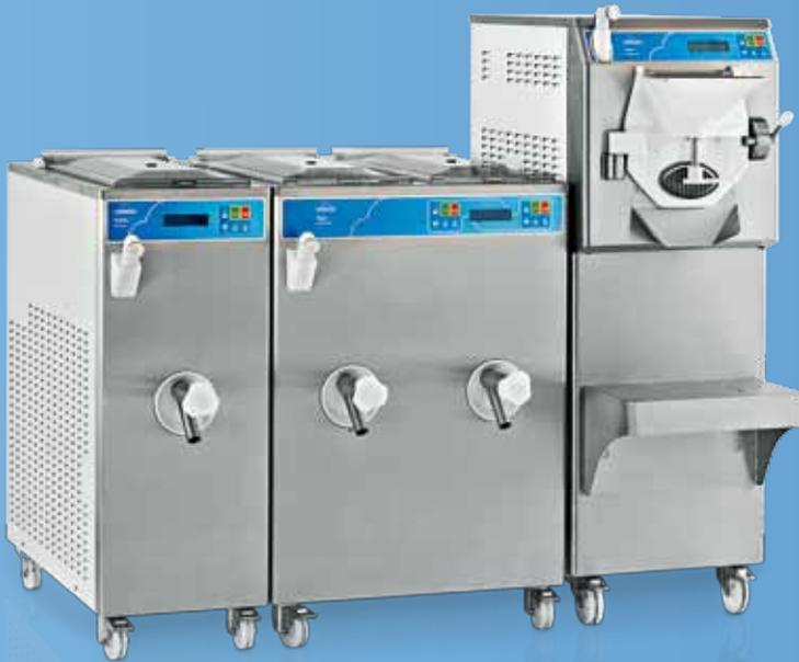
The range of XPL machines, for making artisan gelato is a full range because it includes electronic LABO XPL batch freezers, PASTO XPL electronic pasteurizers and AGE XPL storage/ageing tanks. All Carpigiani machines have been designed and made to comply fully with HACCP international safety and hygiene standards.
