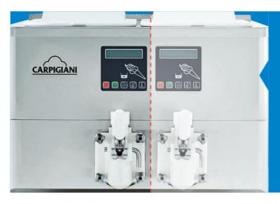
Independent refrigeration system and user interface. Each side runs independently and user can even use just one side if needed.
