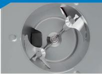
The postponed cleaning program guarantees hygienic safety, by controlling the internal temperature once the product has been extracted. Therefore, it is not necessary to wash the machine immediately in case of prolonged work breaks.
