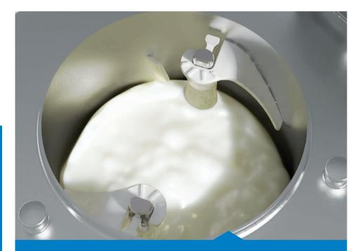
The **stirrer speed** can be modified according to the type of recipe to enhance the intended texture and structure.
