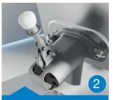
The **second** position: Can clean the tap while maintaining any product inside the machine.
